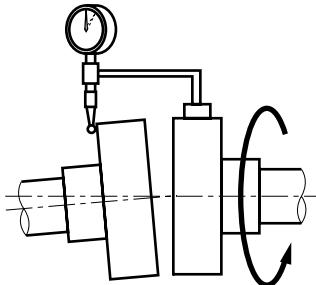
With the indicator set to zero, check the shaft alignment by rotating the shaft and recording the maximum and minimum reading on the dial indicator. This values' difference should not exceed the published value (b-a) for each type of coupling.
