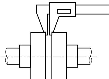
The value read should not exceed the published dimension  $E$  with its corresponding tolerance  $\Delta E$  for each coupling.
