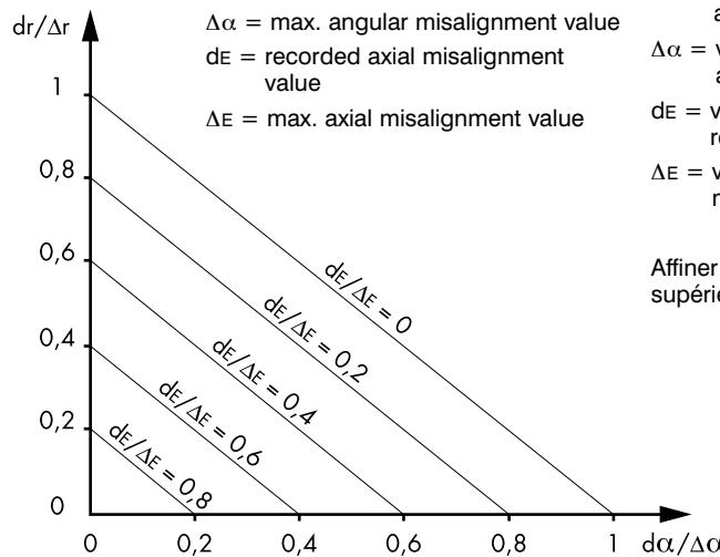
Using the graph above, alignment is correct if the plotted point is found below the  $dE/\Delta E$  desired.
