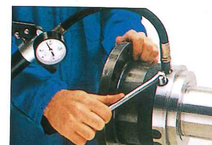
(Step 5) Continue injecting until the manometer shows required value. Tighten the shear tube at a set torque. Calibration chart (Fig. 12) is enclosed with every coupling.
