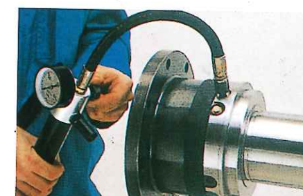
(Step 6) After pressure inside the pump drops, disconnect the pump. Set up the protective plug. Now the coupling is available for use. (These steps take several minutes altogether.)
