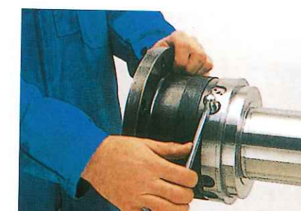
(Step 2) Tighten a new shear tube at a set torque so that the tip of shear tube is fixed on the seating surface.
