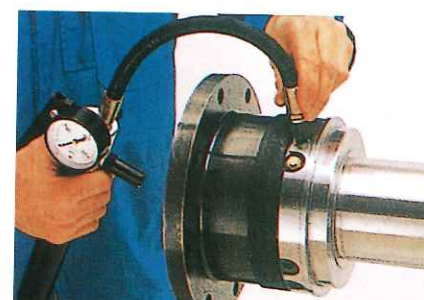
(Step 4) Connect a pump, and turn the shear tube by 1/8 revolution (a channel in the oil filler joint will open).
